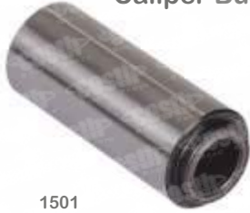
1501 Guide Pin (short) Ø32 / 80 mm
